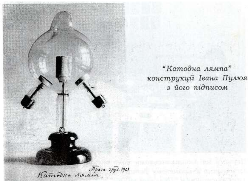
Fig. 1. A cathode lamp designed by Ivan Puluj is a pivotal invention that significantly contributed to the development of X-ray technology.
